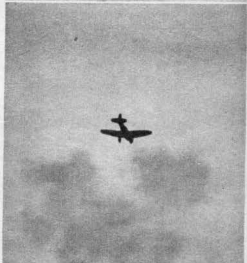
Short nose on Oscar ( above and below ) is its most striking recognition feature. Fuselage by contrast seems long and slender as wing is set far forward. Oscar is an Army fighter, used mainly in the Burma-India theater. The Mark II has a new engine, span 2 ft. less and blunter wingtips.
